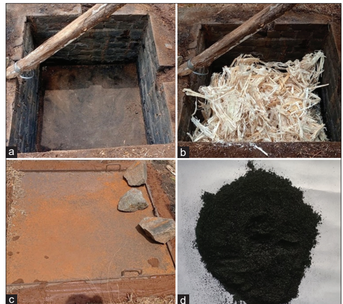
Figure 1: Process of biochar preparation: (a) Kiln used for biochar preparation, (b) Kiln filled with sugarcane bagasse, (c) Closed kiln during pyrolysis process, (d) Sugarcane biochar.
