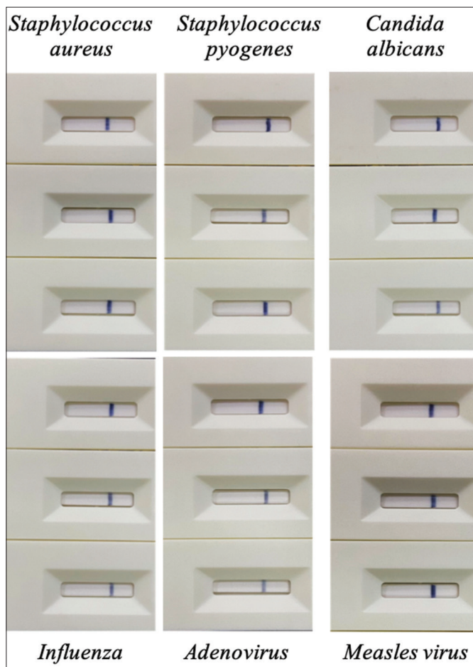
Figure 12: Cross-reactivity of the test strip with potential interfering microorganisms: Staphylococcus aureus , Staphylococcus pyogenes , Candida albicans , Influenza , Adenovirus , and Measles virus .
