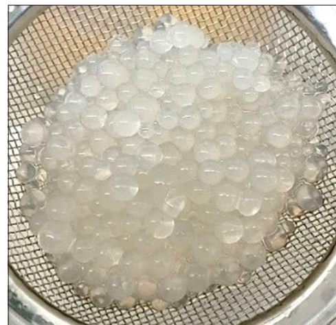
Figure 2: Agar beads embedded with G. subterraneus Tm6Sp1 formed with 3% w/v agar bacteriological and cold mineral oil.
